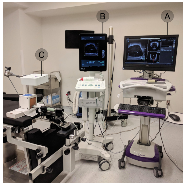
Fig. 1. Clinical setup: A) prototype navigation and dose-planning system, B) ultrasound system, C) EM field generator-tracking system.
